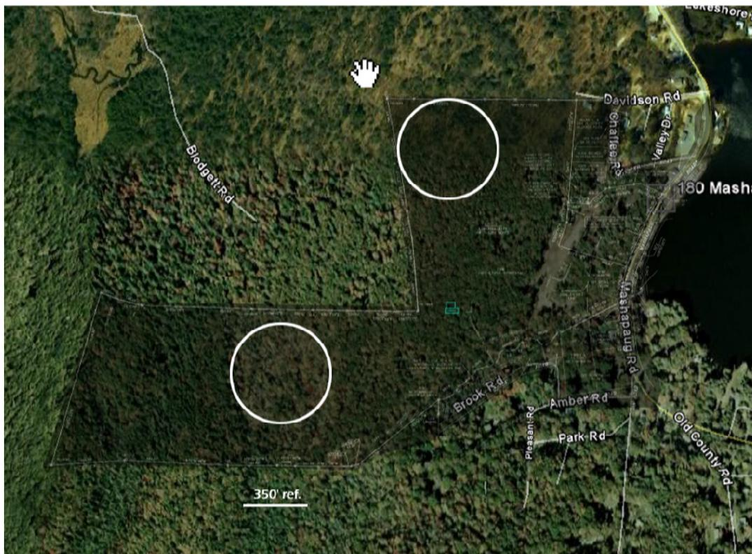
Composite image from Google Earth and Assessors map. Circles indicate potential 700' 'clear zones' for wind turbine placement (750 kW turbines)
